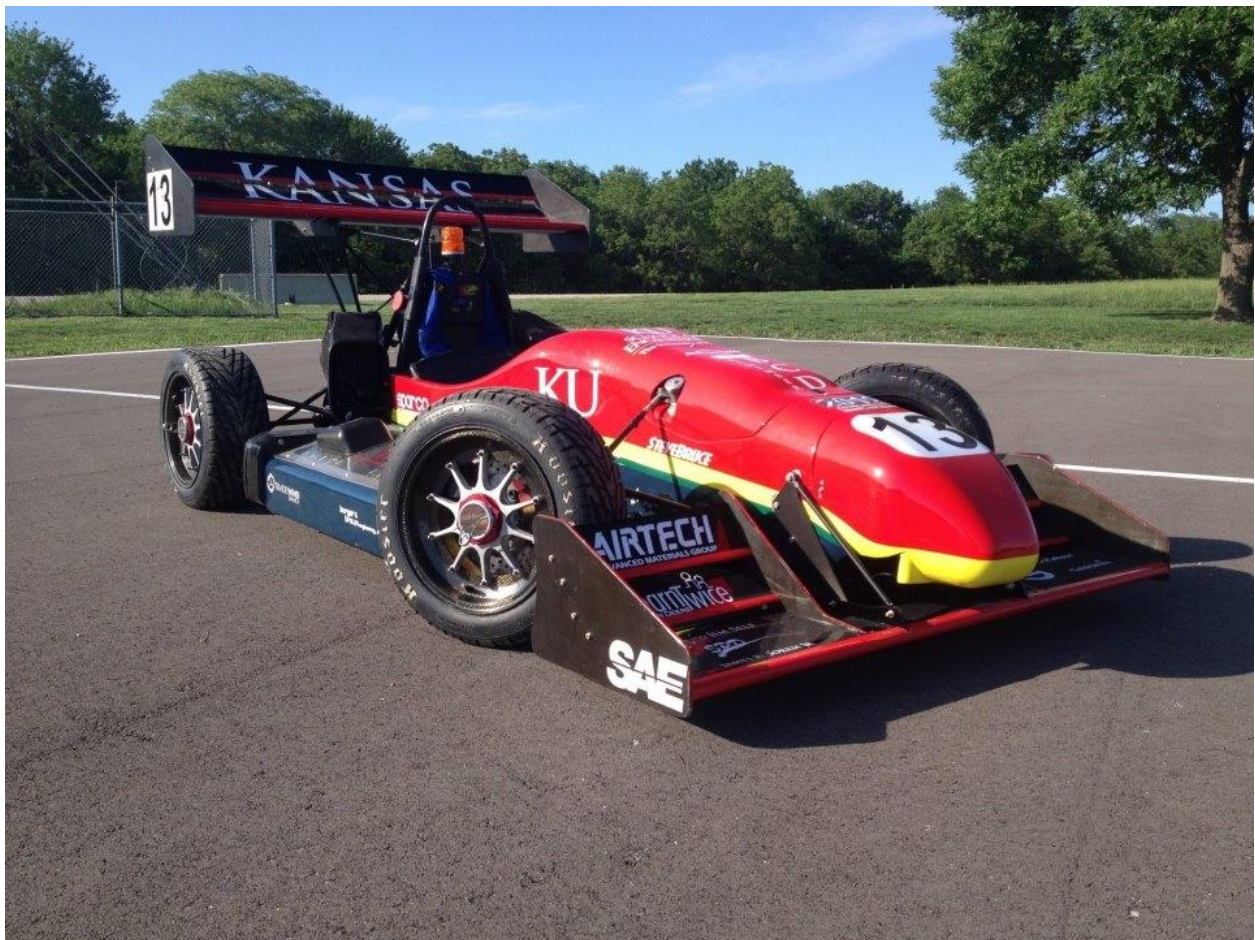
Formula - Direct drive rear axes with EMRAX motors, May 2012
