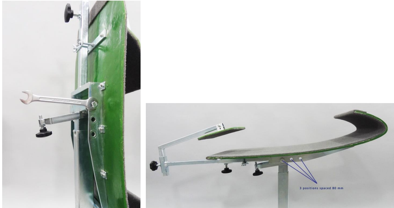
Figure 6: Manually adjustable horizontal cradle position - 3 positions spaced 80 mm
