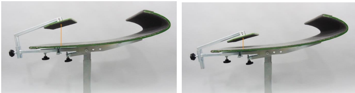
Figure 9: Manually adjustable wing clamp for different thickness of the wing
