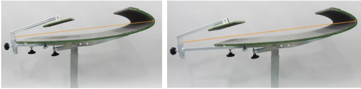
Figure 8: Manually adjustable wing clamp for different chord lengths of the wing (up to 100 cm)
