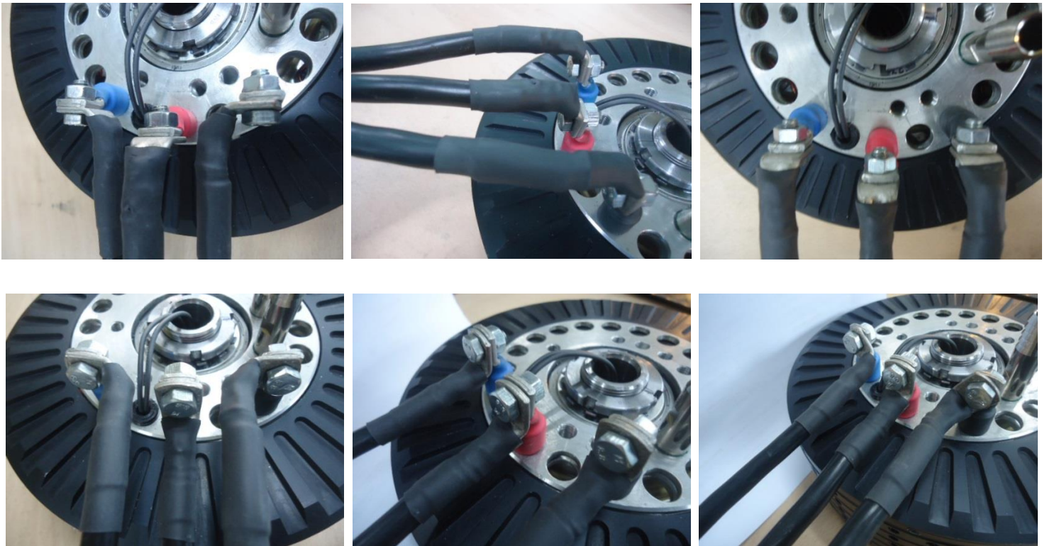
Figure 44: Angular connection of motor connectors to controller cables. Connection must be isolated with shrink hose!
