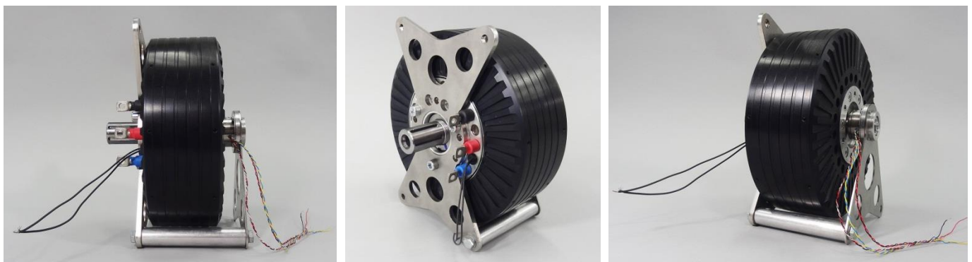
Figure 10: Motor with extended shaft from back motor side
